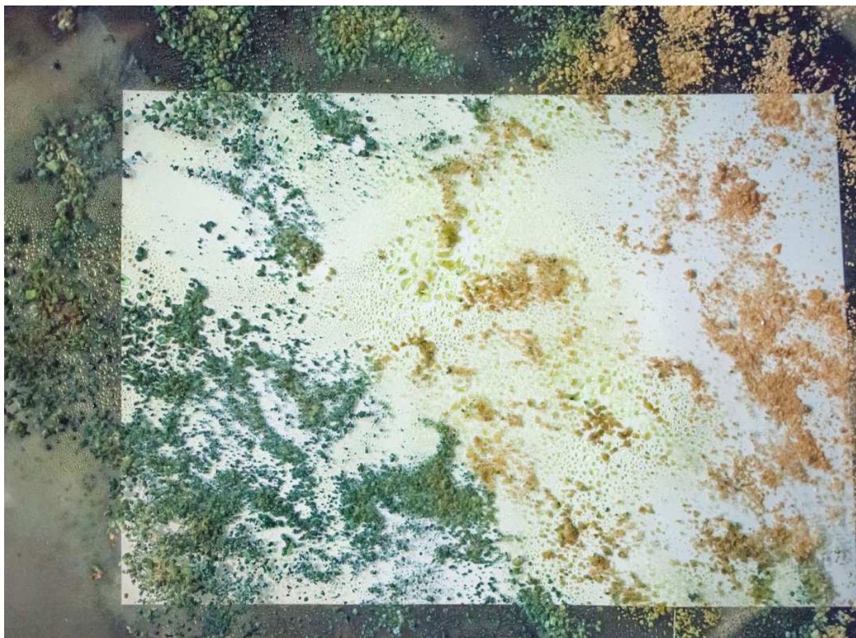
Figure 12: Salt sample from experiments 3.6a and 3.6b. The sample was partly shaded to show the photolytic reduction of iron (III) to iron (II) by spraying potassium hexacyanoferrate (III) on the sample, which forms Prussian blue pigments with iron-(II)
